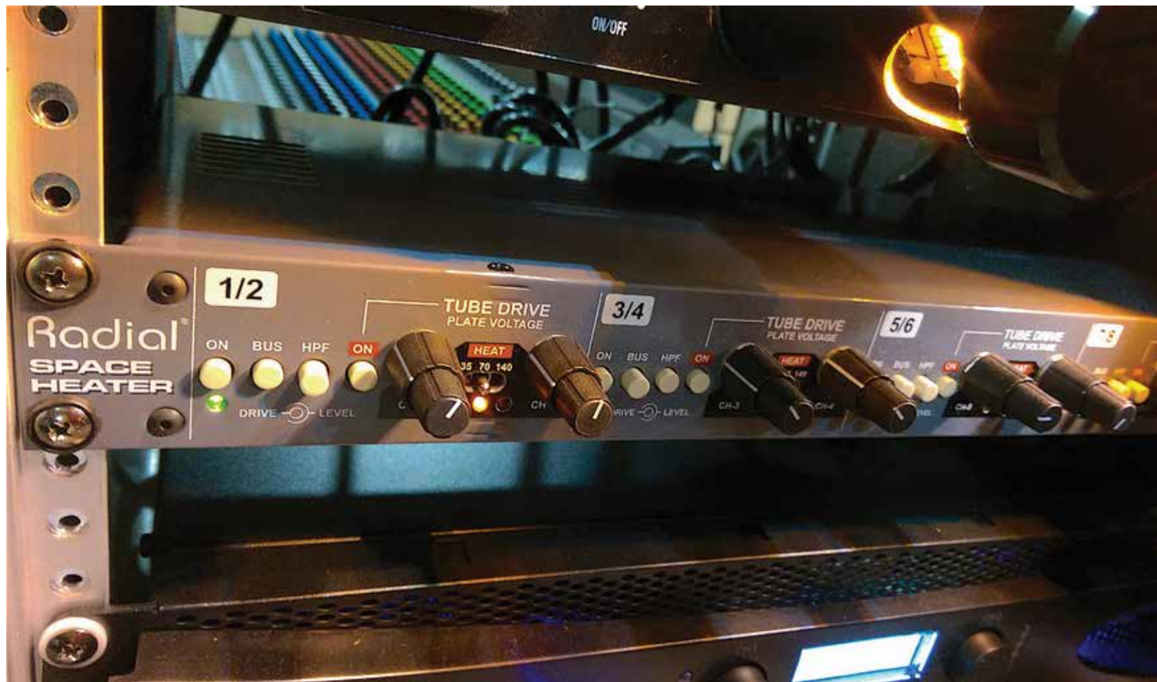
The Space Heater's eight paired input channels each feature variable Drive (level to the tube drive circuit), Level (output level from the tube drive circuit), and three switchable Heat settings that change each stereo pair's tube voltage between 35, 70, or 140 Volts.
