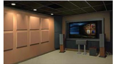
Primacoustic paintable acoustic tiles blend into the room color scheme.
