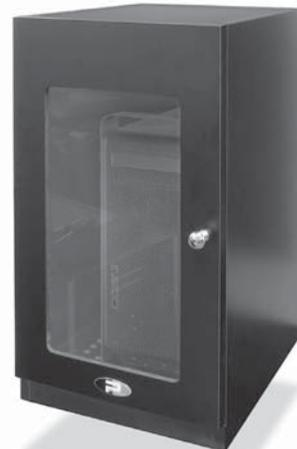
The Machine Room is a fan-cooled enclosure designed to quiet down computers in recording studios. It features heavy MDF construction to add mass and retain sound. To reduce inner reflections, high density open cell foam with embedded fire retardant lines the insides. A unique manifold is employed to reduce computer and fan noise from exiting the Machine Room. A variable speed fan provides the user with control over air flow and desired cooling level. Ships flat, target retail price \$699.
