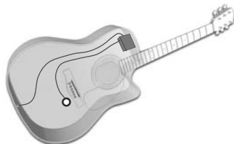
Piezo element wired to battery powered preamp.
