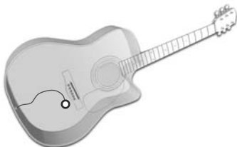
Piezo element wired directly to output jack.
