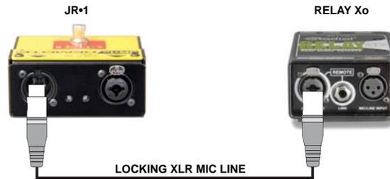
Another advantage is that XLR cables can be daisy-chained together to make a longer cable. This means you won't have to depend on a specific custom built cable to connect your remote device.
