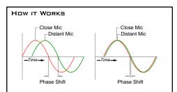
By altering the phase (or delaying the sound) of the nearest microphone, you can shift the fundamental frequency so that it will more gracefully combine with the sound being captured by the second microphone.
