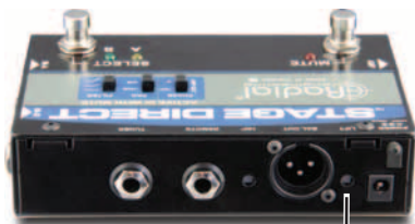
Recessed ground lift switch for the XLR output located on the rear panel.
