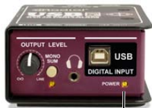
LED Power Indicator
