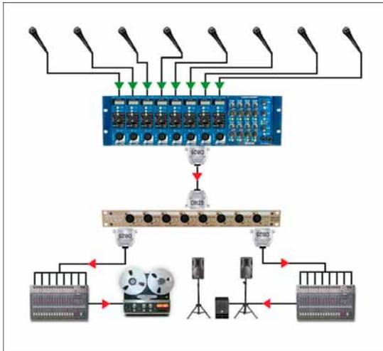
**Using the LX8 to feed two different audio systems**
