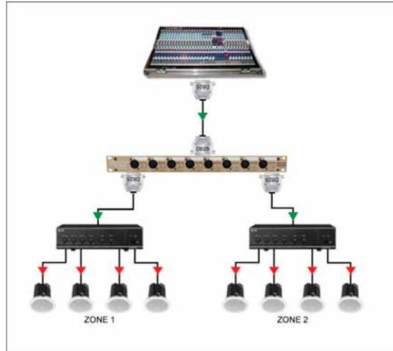
The Radial LX8 features an internal grounding option that will be of interest to system engineers when integrating the LX8 into complex audio-visual systems.
