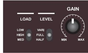
Set both 3-position switches to their middle position. This will disengage the GAIN control and provide maximum boost to your mic signal, while setting the load to a good starting point for experimenting.
