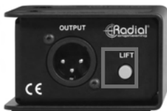
The Lift switch
